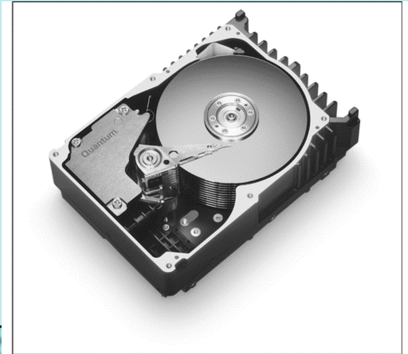
Figure 1-17 Hard drive with sealed cover removed
